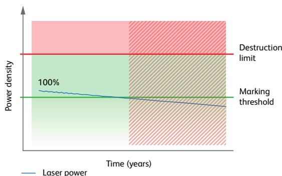
As an example, typical specification for a Videojet 30W laser is an 80% setting which equals to 24W.
