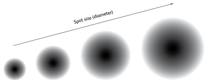
The spot size is determined by the combination of marking head aperture (6, 10, 12mm) and lens. The laser 'power' is distributed over the spot's area which results in a certain 'power density' for a given laser power and the spot size. It is important to understand that the spot's area increases with the square of its diameter. Consequently, if the spot size is increased by a factor of two, the power density is reduced by a factor of 4 (down to a quarter).
