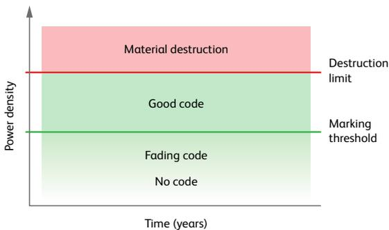
Power density below the marking threshold may result in weak or faded codes, however, increasing the power density too much could exceed the second threshold (destruction limit) and potentially damage the material. Only if the right amount of power density is applied, will consistent, high contrast codes be achieved.
