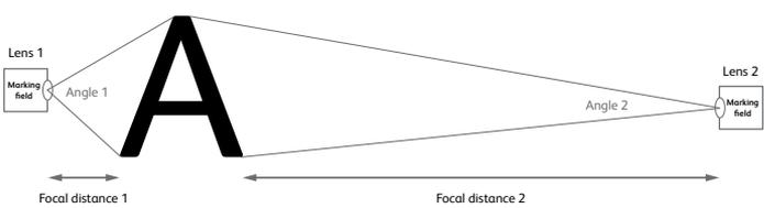
Therefore a marking head using larger focal distance lenses will show a substantially higher performance than using small focal distance lenses. The downside here is that the larger focal distance will result in a larger spot diameter which in turn requires increased laser power.
