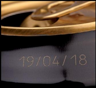
The second important factor influencing the power density is the marking speed - the speed at which the marking head scribes the lines forming characters or other symbols.
