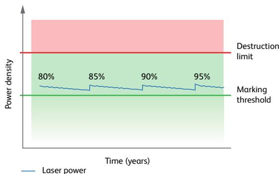
To compensate the loss of power and assure that even after 5-7 years of operation the laser is still fully capable of achieving the desired performance, all initial marking tests should be done with less than 100% output power. This allows additional power to be available for adjustment over time.
