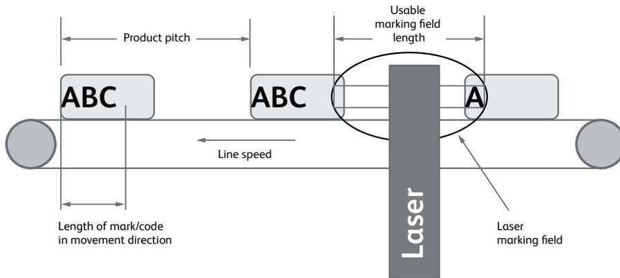
The picture opposite shows a row of products moving right to left. The oval area demonstrates the mark field, sometimes referred to as the mark window, i.e. the window of opportunity where the laser can mark on the product. The optimal combination between mark window and production line is achieved when the mark window can be used to its maximum. That is the case when:
