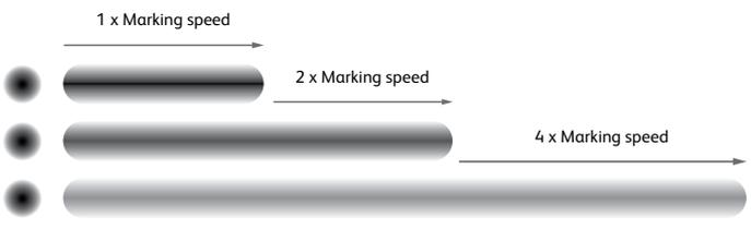
The power emitted by the laser is spread over an area forming a line. If the marking speed is doubled, the area will double that is covered by the laser beam in the same time. Hence the power density shrinks to half. Similarly, if the marking speed is increased by a factor of four, the power density will shrink to a quarter.
