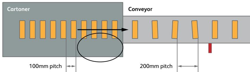
**Picture above:** Best mounting position is inside the cartoner (oval circle) as the product to be marked is guided. In contrast, marking on the conveyor belt (although seems the most obvious) induces the risk of product movement and hence possibility of lower mark quality.
